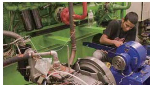
Combustibility test of biodiesel fuel in Bandung Institute of Technology (SEED-Net Project)
